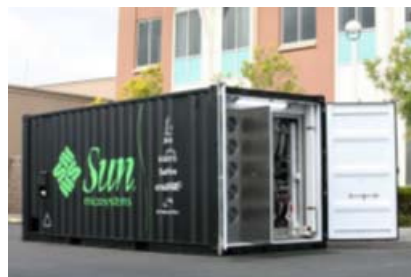
Containerized Data Center
